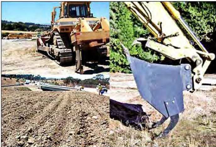
Figure 5. 16 Soil aerator implement
