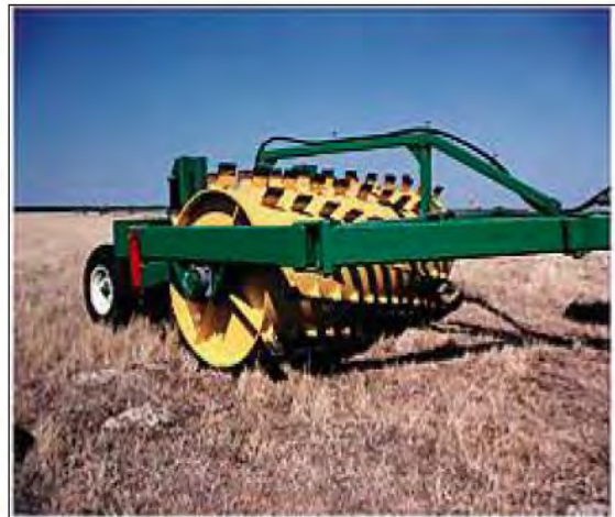
Figure 5. 17 Soil aerator implement
