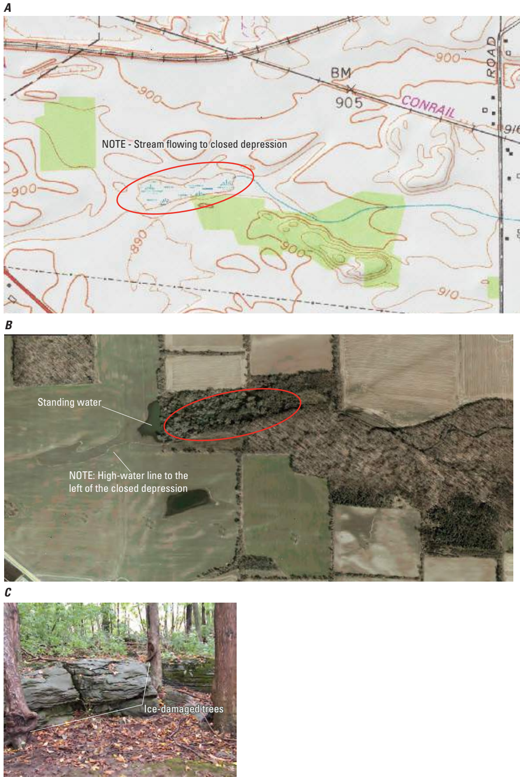
Figure 3. A closed depression near Batavia, Genesee County, New York, from A , a part of a 1:24,000-scale topographic map and B , a Google Earth image showing a closed depression (red ellipse) and C , the interior of the closed depression where surface water infiltrates into the Onondaga Limestone. The high-water line is shown to the left of the wooded area and standing water adjacent to the woods. Tree ‘scars’ ( C ) appear where ice formed when the depression was filled with water and the ice damaged the bark layer of several trees.
