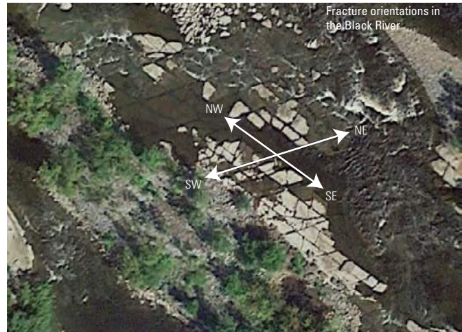
Figure 10. Draining of a surface-water holding pond in Watertown, New York. A , Bedrock fracture found below approximately 6 feet of glacial clayey soil in which the holding pond was located; B , solution opening along this fracture where surface water drained to groundwater; C , orientations of primary bedrock fractures in the Black River, southwest of the holding pond and east of the New York State Route 12 bridge in Watertown.
