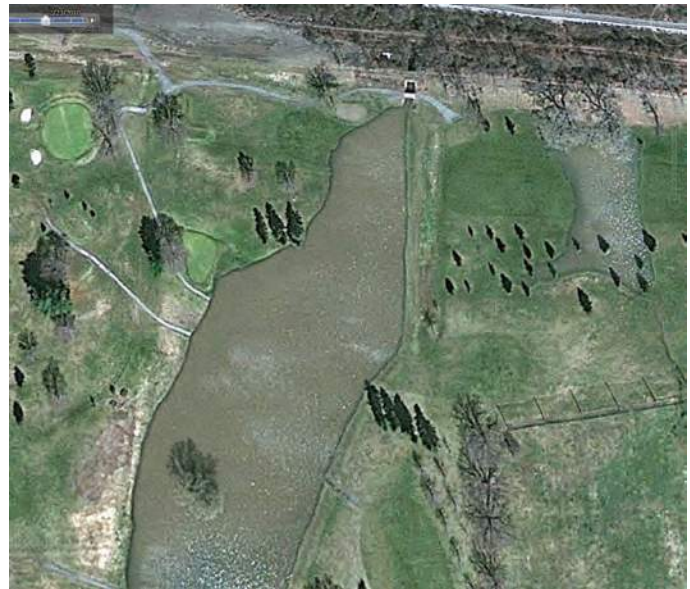
Figure 8. A closed depression (sinkhole-swallet) in Onondaga Limestone at the LeRoy Country Club in LeRoy, Genesee County, New York, in A , March 2010 and B , September 2013. Surface water contributed from a shale bedrock watershed to the south of this view. In March 2010, the depression was filled with surface-water runoff and had a karst water table above land surface, whereas in September 2013, the karst water table was below land surface.
