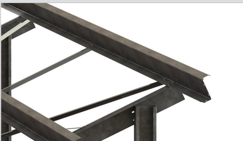
Galvanized purlins with large wire management tray
