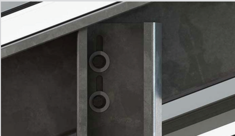
Slots enable vertical adjustability
