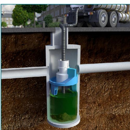
Fig.3 Maintenance is done with a vacuum truck
